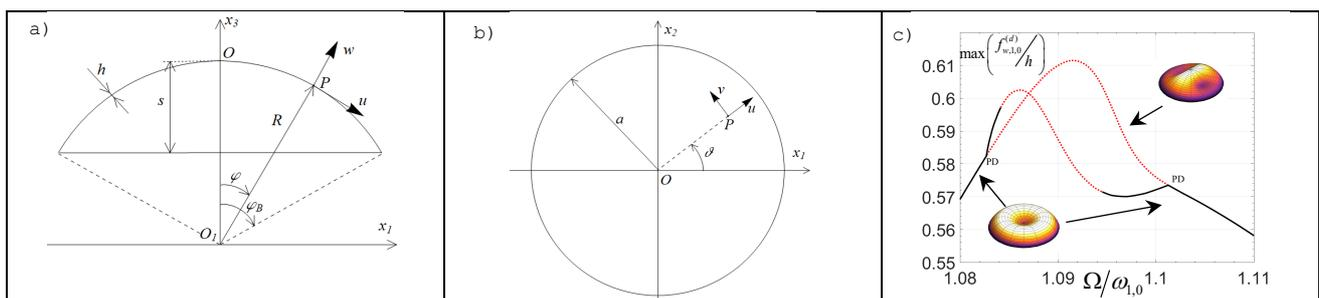
Figure 1: Geometry of the cap, a) lateral view, b) top view. Amplitude frequency diagram c).
