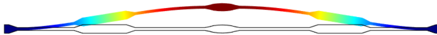
Figure 1: The fundamental vibration mode of a clamped-clamped beam with an optimized shape. The color denotes the displacement. The mode shape is obtained by using COMSOL Multiphysics 5.4 with 2D solid element.
