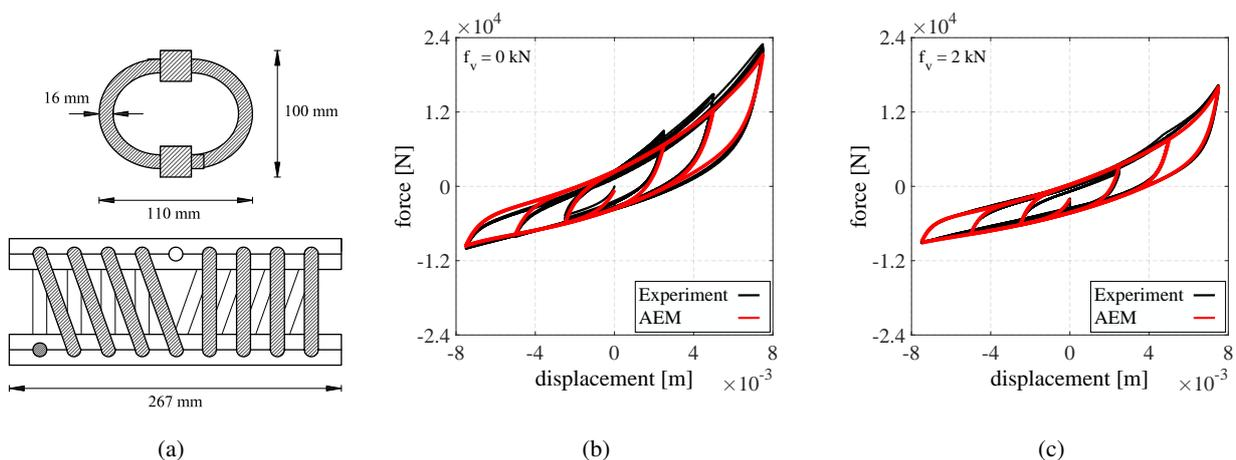
Figure 1: Comparisons of analytical and experimental results obtained for the tested WRI (a) in axial direction without (b) and under (c) the effect of an axial compressive preload  $f_v = 2$  kN
