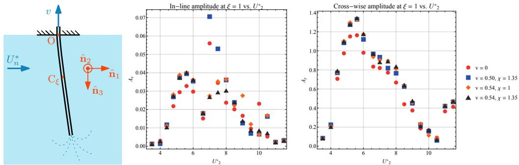
Figure 1: Schematic representation of a submerged cantilevered flexible pipe aspirating fluid and the in-line and cross-wise amplitudes of the oscillations of the center of the inlet section of the pipe as a function of  $U_2^*$  for all the analyzed scenarios.
