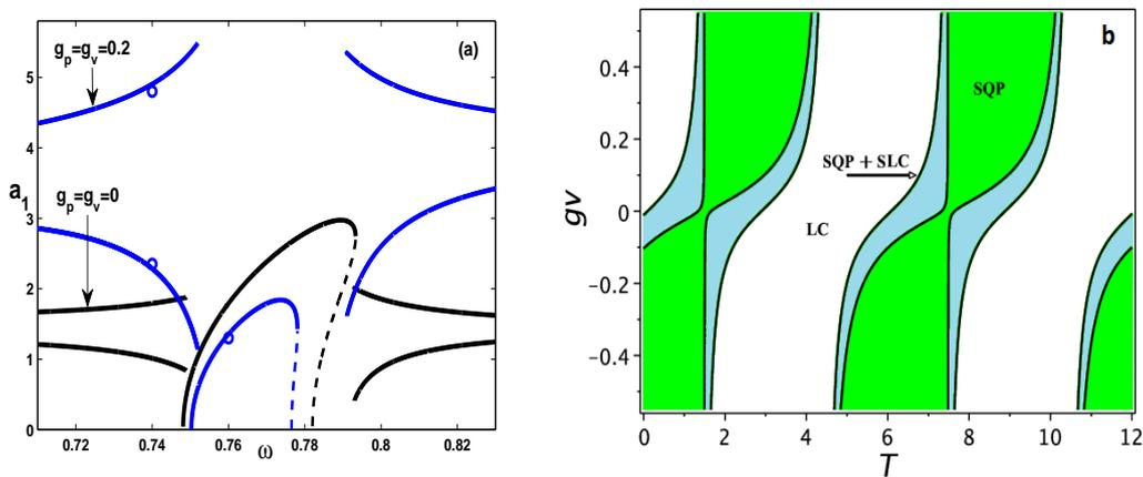
Figure 1: (a) Frequency-response curves near the first natural frequency for  $T = 3$ ,  $g_v = g_p = 0$  for black line,  $g_v = g_p = 0.2$  for blue line. (b) Stability chart in the plane ( $g_v, T$ ); (LC) limit cycle, (SQP) stable QP, stable LC (SLC) for  $g_p = 0.1$
