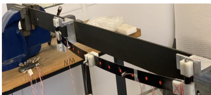
Figure 1: Photographic view of a lab set-up of a coupled two-beam system, with at least three equilibrium states, instrumented with eight accelerometers, five in the core beam and three in the attached continuum, to sample the transversal acceleration field. Right figure: the space distribution, POD modal shape, of the 1 st principal acceleration signal is localized over the domain of the multiple-equilibria continuum (red thick line).
