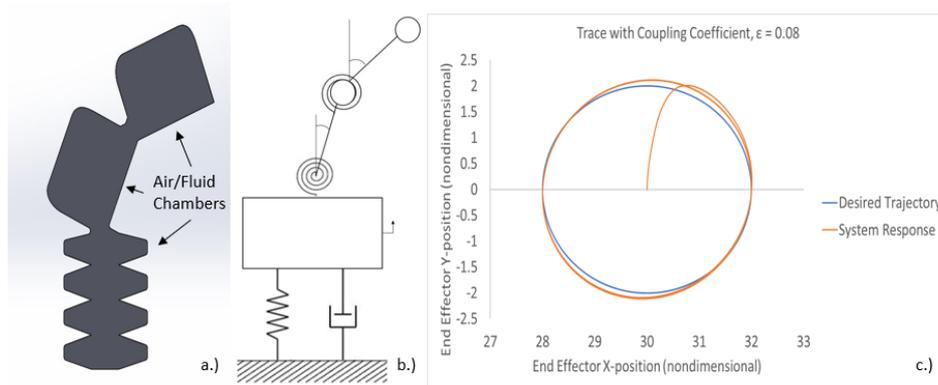
Figure 1: Figure 1: a.) Physical System, b.) Dynamic Schematic, c.) Circular Trajectory
