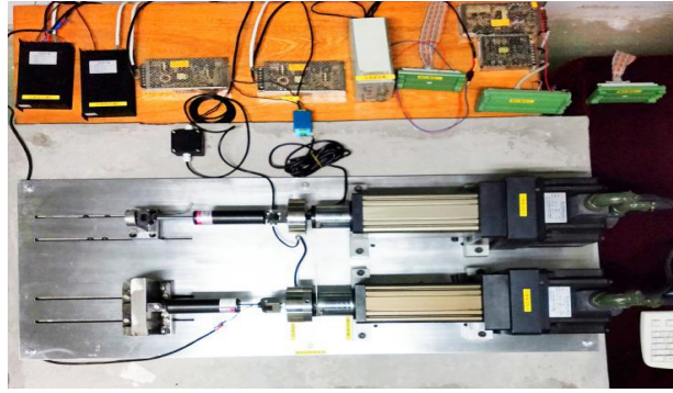
Fig.3 Hardware in the loop test of MR dampers
