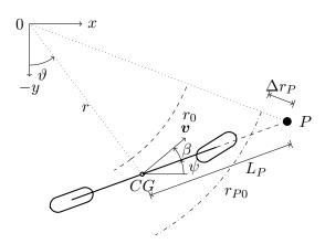
Figure 1: Geometric relations for the driver's preview model: To follow a circle with radius  $r_0$ , the driver spots a point Pat a distance  $L_P$  straight ahead of the vehicle, which should move along a circle with radius  $r_{P0}$ .
