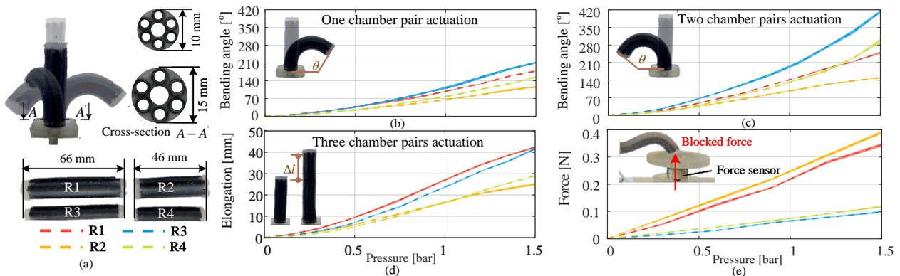
Figure 1: Characterisation results. (a) The designed four robots (R1-R4) and its cross-sectional geometries. The results for (b) one chamber pair actuation (c) two chamber pairs actuation (d) three chamber pairs actuation and (e) tip force generation.
