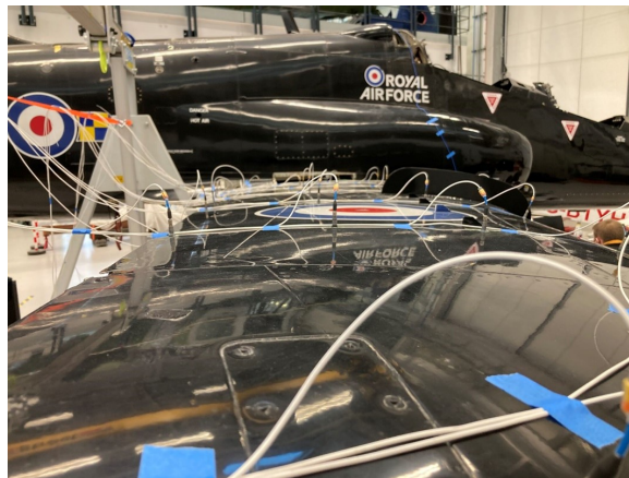
Figure 1: Experimental setup for the vibration testing of the Hawk T1A Wing
