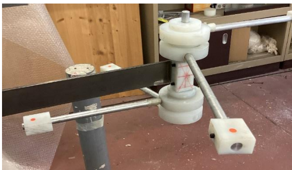
Figure 1: Lab set-up of conceived physical meta-structure (NTUA Nonlinear Dynamics Lab Unit) to explore experimentally dynamics underlined by irreversible energy flow from an elastic beam into an interacting stack of coaxial eccentric rotors in contact with stators. Observation: the tangent acceleration component of the eccentric masses is a strictly positive quantity with pulse-like behavior (right) during energy flow. Interplay of geometric nonlinearities and polygenic nonlinear contact-induced friction.
